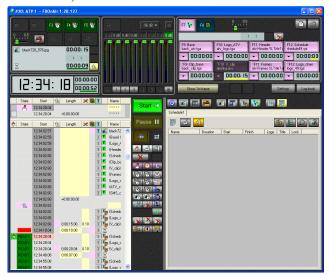
The FDOnAir application is designed to control broadcasting in an automatized way i.e. schedule preparation (play-list), broadcast realization, broadcast control and its adjusting.
