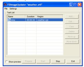
FDImageUpdater program is designed for dynamic change of graphic files. FDImageUpdater output information is updated during broadcasting e.g. temperature, pressure, humidity.
