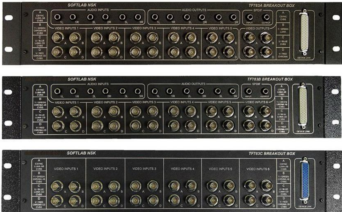
Figure 93. The front view of the breakout boxes for connecting several FD300 boards
