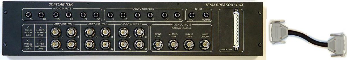
Figure 89. The appearance of the passive breakout box with the connection cable
