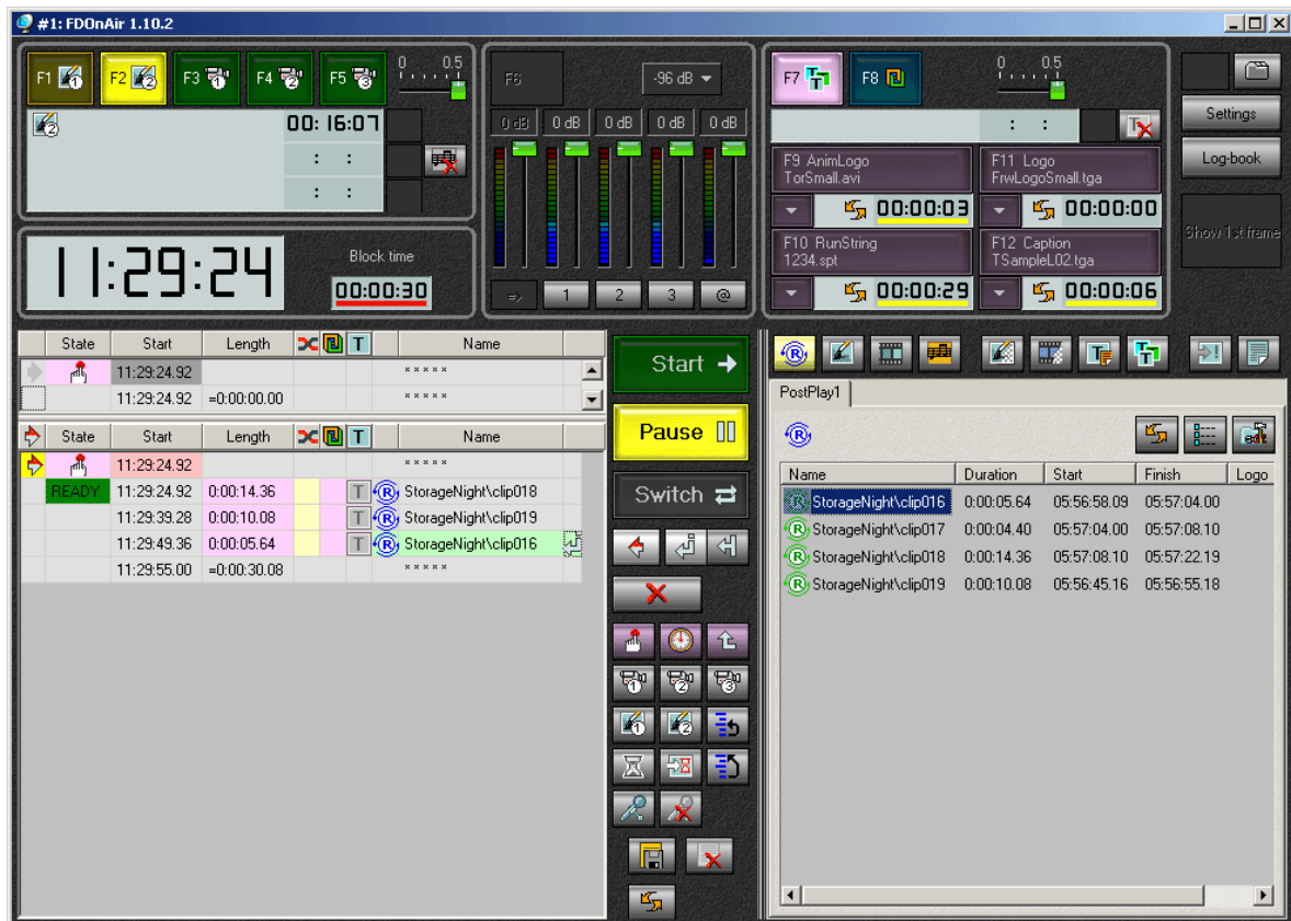
Figure 42. The FDOnAir application main window with PostPlay clips list and a schedule
