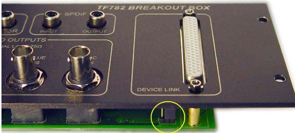
Fig. 12. Location of the grounding contacts on the passive breakout box
